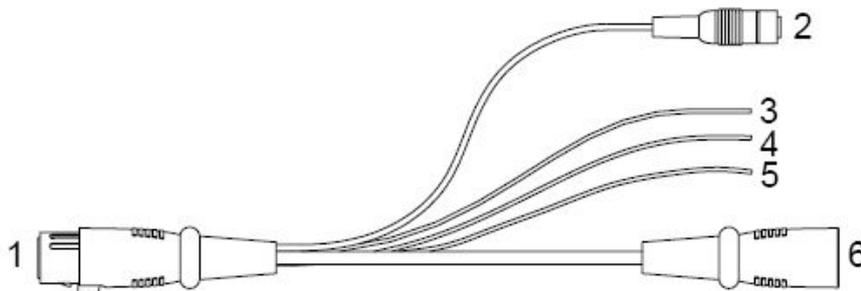
1. XLR (M) connector: to connect the XLR connector on device.
